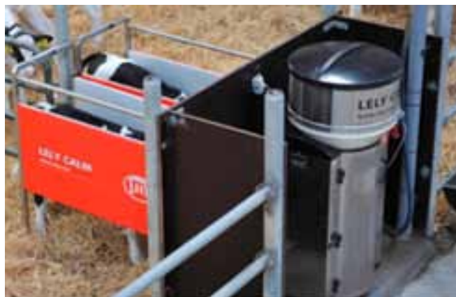
This automated feeder used for calf rearing measures out portions tailored to the individual calf, triggered by the EID worn by each animal. The deer industry could also use EID as a basis for smart technologies to improve productivity, says Kim Kelly.
