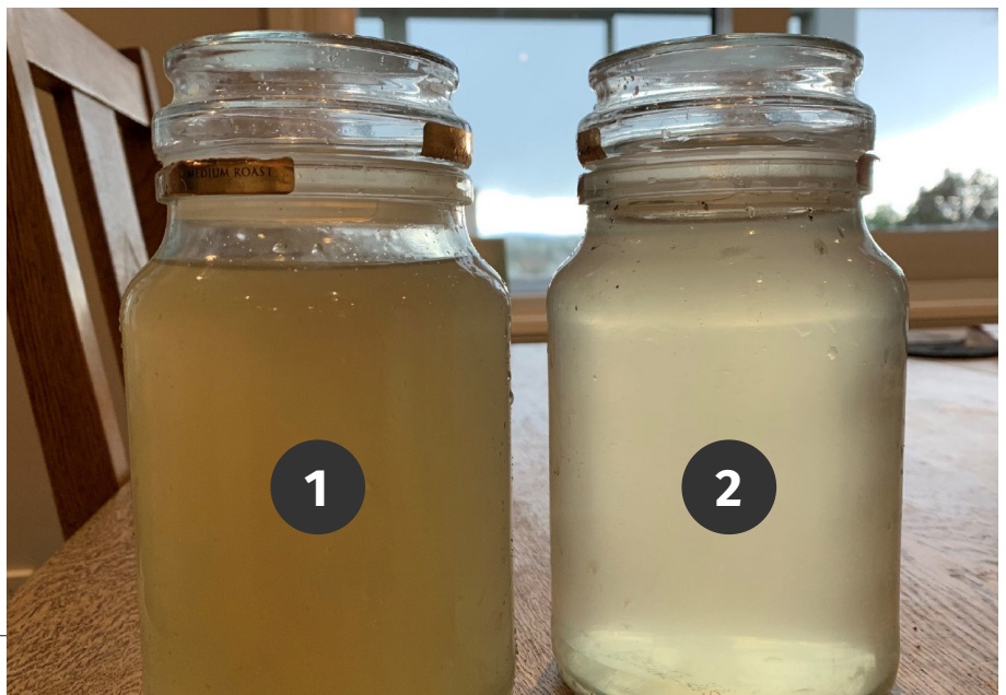
1 Water entering sediment trap 2 Water leaving sediment trap
