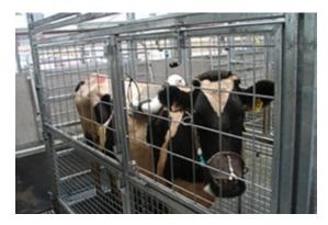
Dairy cattle fitted with  ${\rm SF_6}$  apparatus for Methane measurements
